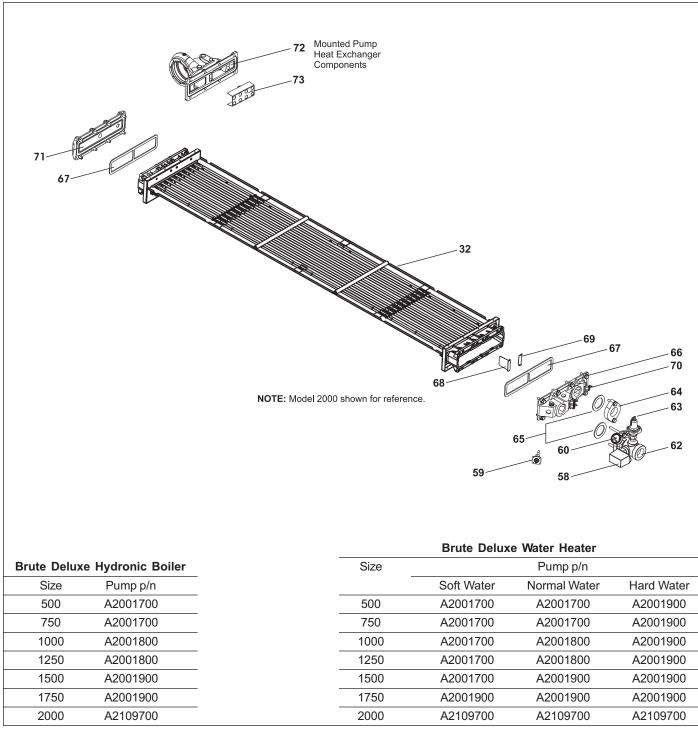
Figure 25. Heat Exchanger Components.
